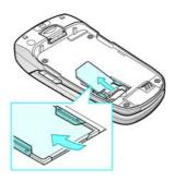
4. Place the battery back, taking care to match the tabs on the battery with the grooves on the phone.
