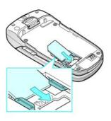
**Note:** When you need to remove the SIM card, slide it, as shown, and take it out of the socket.
