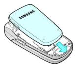
5. Press the battery down until it clicks into place. Make sure that the battery is properly installed before switiching on the power.
