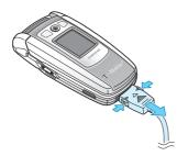
**Note:** You must unplug the charger before removing the battery from the phone during charging; otherwise, the phone could be damaged.
